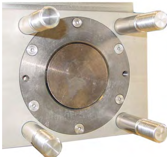
Extruder plate dismantled
